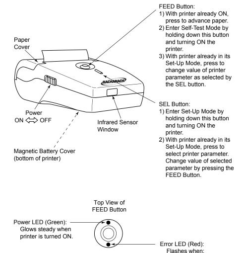
Figure 1. Component Locations and Functions
