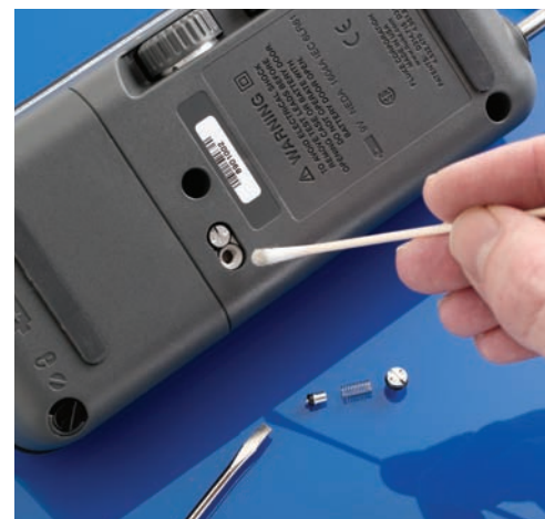
Cleaning the fluid trap in the Fluke-718 Calibrator is quick, easy and only requires a slotted screwdriver and cotton swab
