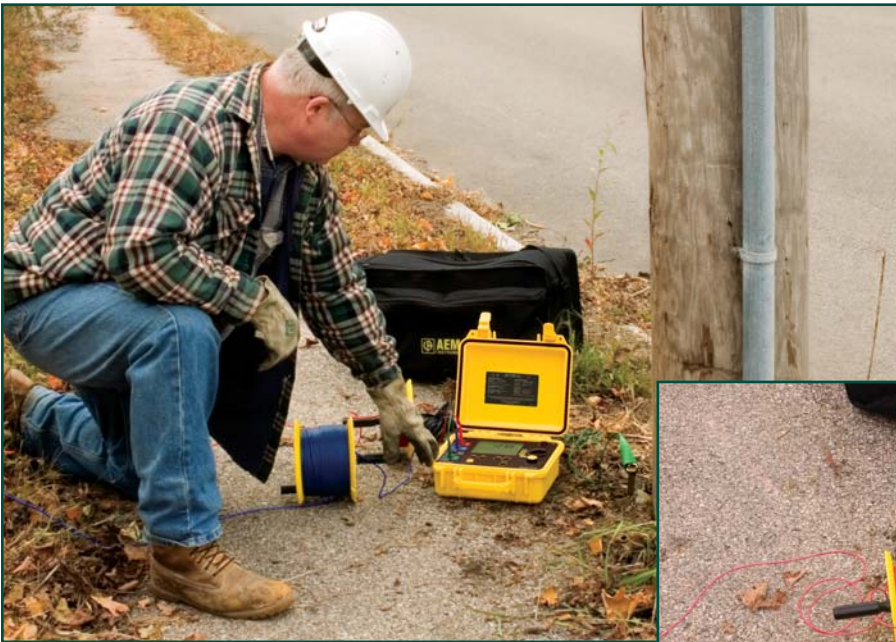
Model 6470 quickly checks ground rod resistance with its Connect – Press – Read approach
