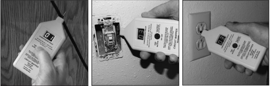
3. If direct conductor contact is not possible, the Receiver has a built in amplifier that can read through most electrical wiring insulation. Hold the square Receiver tip (not prong) against the insulated wire to be tested. Push and hold the ON/OFF button until a reading is indicated. Continue holding button for an additional two seconds to verify a single circuit reading.
