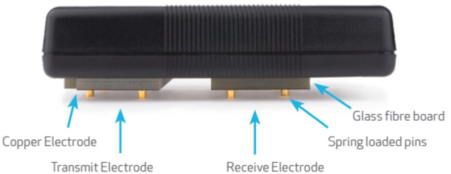
This field penetrates the material under test. A very small alternating current flows through the field. The CME4 detects this current, determines its amplitude and converts it to a moisture content value. By simply pressing the CME4 down on the surface in strategically chosen locations, instant readings can be taken over a large area.
