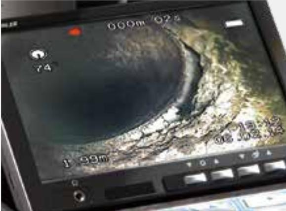
The "Save function" makes it possible to save and view what you see at the push of a button. The integrated position indicator ensures you keep your sense of orientation in the pipe.
