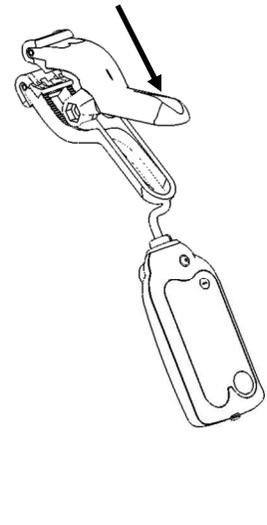
Utilize flexible strap to tightly secure strap clamp to pipe surface where temperature measurements are desired.
