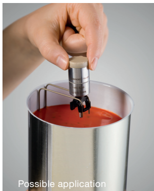
Temperature measurement in a can: testo 191-T1 + stand
