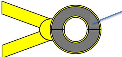
The iron core will have wire wrapped around it in order to transfer an AC signal. However, a DC signal will magnetize the iron core.
