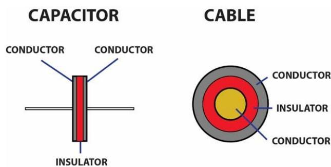
The longer a cable is, the greater the surface area of its conductors and the higher its capacitance will be.
