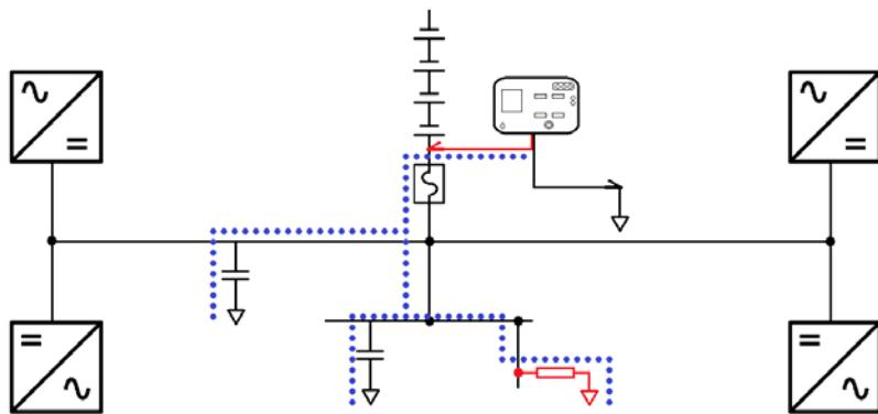
Therefore, if you do not know which circuit has the real fault and which circuits are only drawing current due to capacitance, then you can be tracing the wrong path all day and never find a fault.
