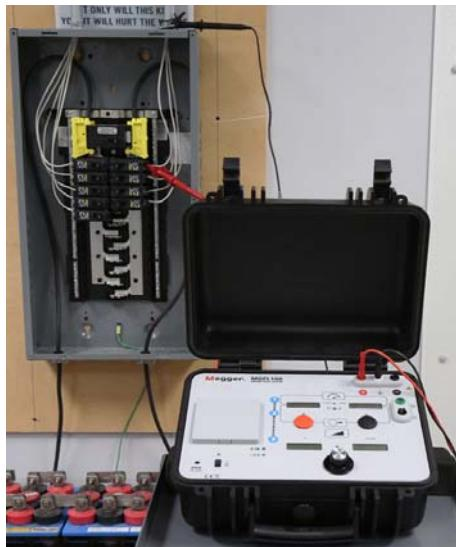
Turn on the MGFL100 output and apply a small current through each circuit. The transmitter will display the resistance and capacitance of each circuit.
