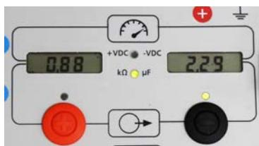
Some of these circuits would be expected to read OL, with very high impedances. When a fault occurs, use the transmitter to read the impedance of each circuit and compare them to the un-faulted impedance. This can help you locate the circuit that has changed and has the fault.
