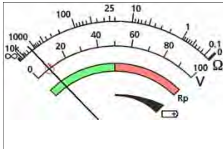
Figure 16: ground noise voltage indication
