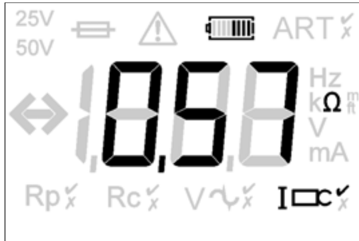
Figure 36: example resistance reading using two-clamp stakeless method
