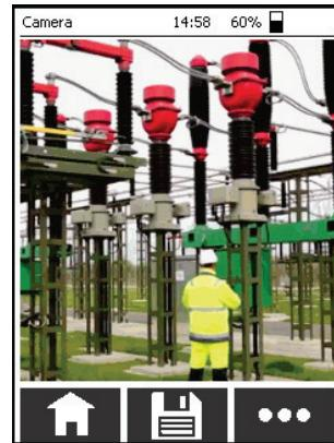
If the green cross indicating which can be enabled /disabled (see page 50) appears in the centre of the screen, it should be positioned as precisely as possible on the identified problem area or any other point relevant to the measurement when capturing the image. The green mark will then also be visible in the image file afterwards.
