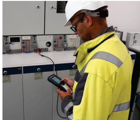
The PD levels themselves are of less importance for this type of measurement. Rather, the PRPD diagram should be checked for typical PD clusters and patterns.
