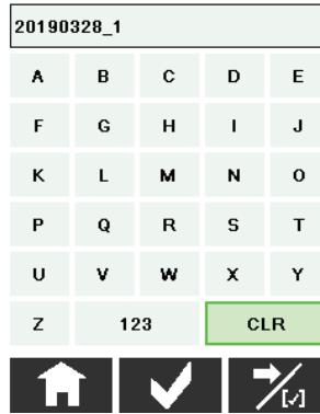
Briefly pressing the button allows the user to scroll through the list of fields on the touch screen. Pressing the button deletes the last character that was entered. Pressing and holding the button deletes all characters. You can switch to the numeric keypad by pressing . In addition to number keys, the keypad also has six freely assignable keys for frequently used text modules.
