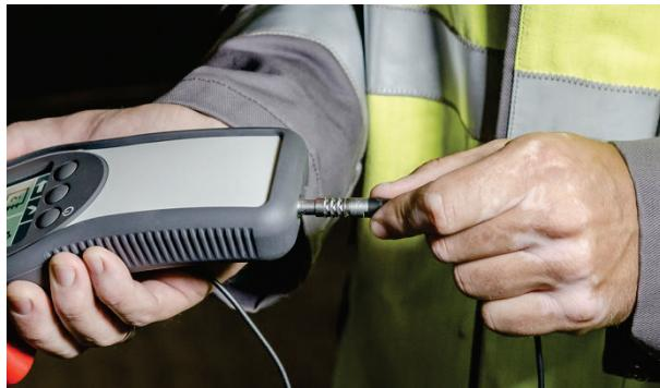
The device automatically detects the connected sensor after being switched on, and offers a choice between the potential operating modes.
