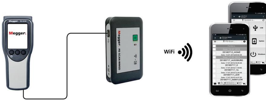
When a PD scan PD Scan is connected to the WMDS, all new measurement data sets are automatically downloaded to the internal memory of the WMSD. This function means that the mass storage device can also be used to collect the measurement data from multiple measuring devices that are in use without having to bring them to the office.
