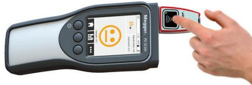
3. Press the push-button on the function tester to generate a PD-like signal.
