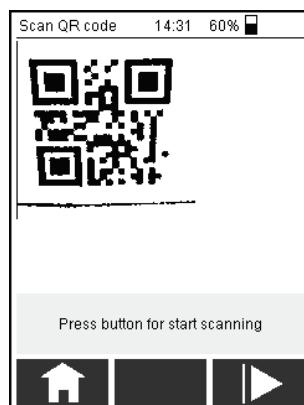
3. Hold the PD Scan up to the QR code and press the button. The integrated camera will now try to read the QR code, and will show its character string at the bottom of the display as soon as it was able to be scanned.
