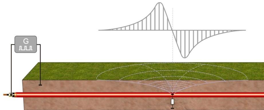
This particular effect is most beneficial for pinpointing sheath faults, by measuring the value as well as the polarity of the step voltage using two earth spikes and approaching the deflection direction following the fault position.
