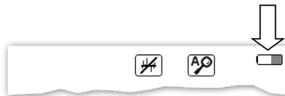
If the bar is barely filled, it is advisable to carry replacement batteries. As of a residual capacity of about 20%, both the battery status indicator and the LED in the
