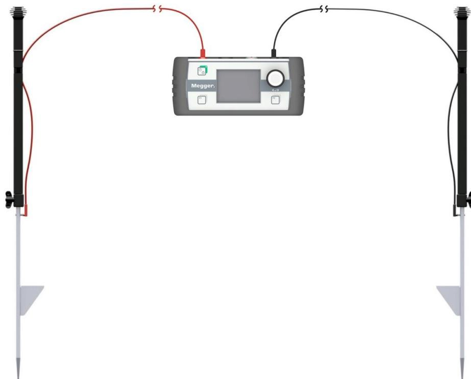
To avoid switching back and forth or even accidentally pulling out the cable while operating, it is advisable to attach the cable to the earth spike as shown in the diagram:
