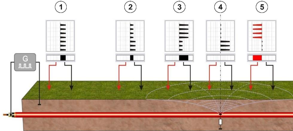
As voltage gradients induced by the current flowing back from the fault position exist around the earthing point of the generator, the measurement values near this point might be elevated (position 1). However, the deflection direction (polarity) also indicates the direction of the fault position at this point.
