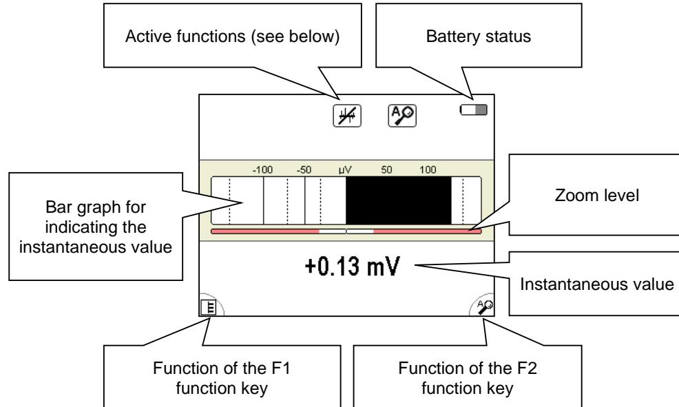
**Active functions and modes** The symbols at the top right of the measurement screen indicate the following functions and measurement modes:
