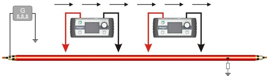
**Distance between the earth spikes** The distance between the earth spikes directly affects the step voltage reading. If the distance increases, the potential difference between the two earth spikes rises and therefore the voltage reading shown on the indicator unit as well.
