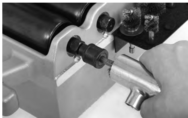
Figure 14 – Nettoyage interne des raccords
