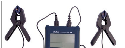
Fig. 18: Connection of the temperature clamps
