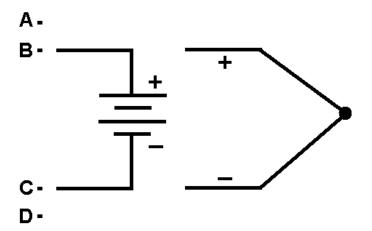
See section 10.0; Technical specifications for supported types of thermocouples. The multi-scanner has a cold junction compensation function. Normally this function should be ON and the actual temperature of the thermocouple can be measured. With CJC OFF, the multi-scanner will measure the difference between the thermocouple at the junction and at its TC input terminal.
