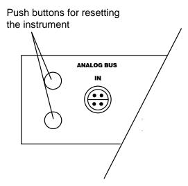
The push buttons on the back of the B-models can only be used to reset the instrument.
