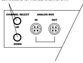
The push buttons on the back of the A-models can be used for manual channel shift. When LED 1 is flashing no channel is selected. These buttons will enable the user to operate the instrument without using a connected computer.
