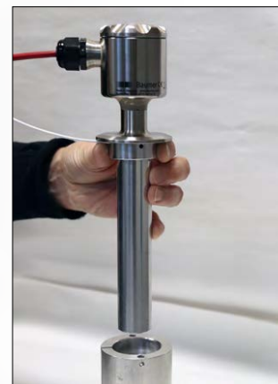
Assembled RTC-156 insert and RTC-158 adapter.
