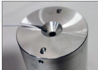
STS-102 A 035 sensor in an insert.
