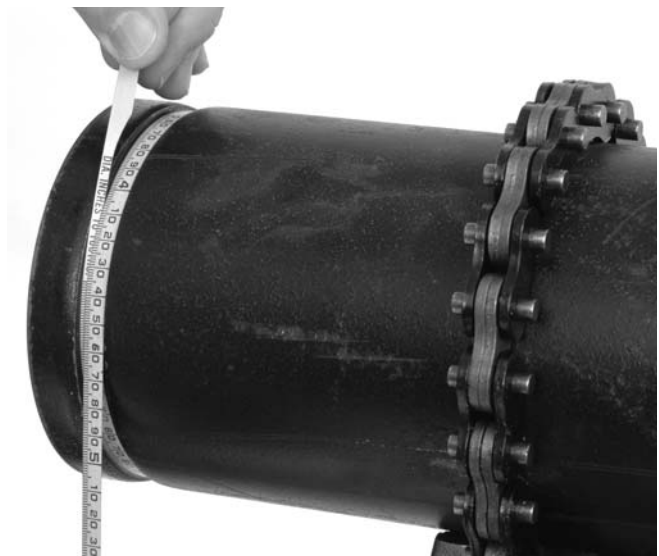
Figure 16 – Measuring The Groove Diameter With A Diameter Tape
