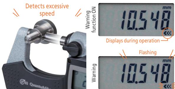
The approach speed warning function detects collisions with workpieces due to excessive speed. The display flashes when this feature is enabled, making it possible for even inexperienced operators to obtain stable and accurate measurement results.
