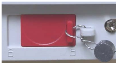
Locked with Wire Seal
