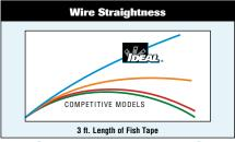
Wire Straightness Test (Blued Steel™)
