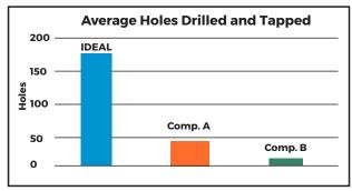
Based on testing 1/4-20 drill tap in 10 AWG Mild Steel
