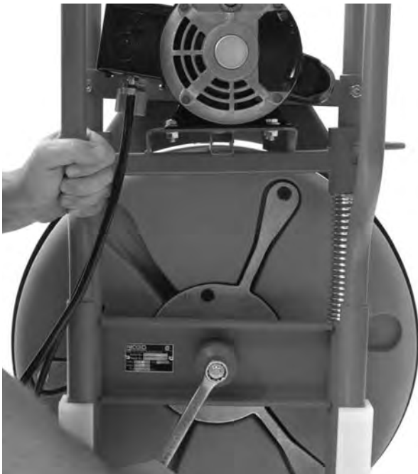
Figure 18 – Removing Drum Bolt
