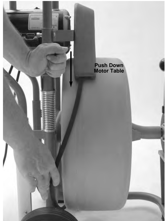
Figure 17 – Releasing Belt Tension
