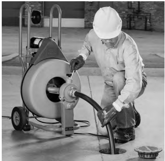
Figure 15 – Using Machine with Guide Hose
