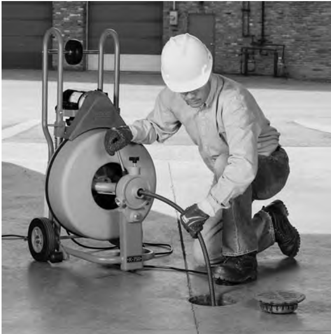
Figure 14 – Operating the K-750 using the AUTOFEED
