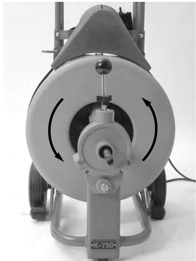
Figure 8 – Proper Drum Rotation (FOR Switch Position)
