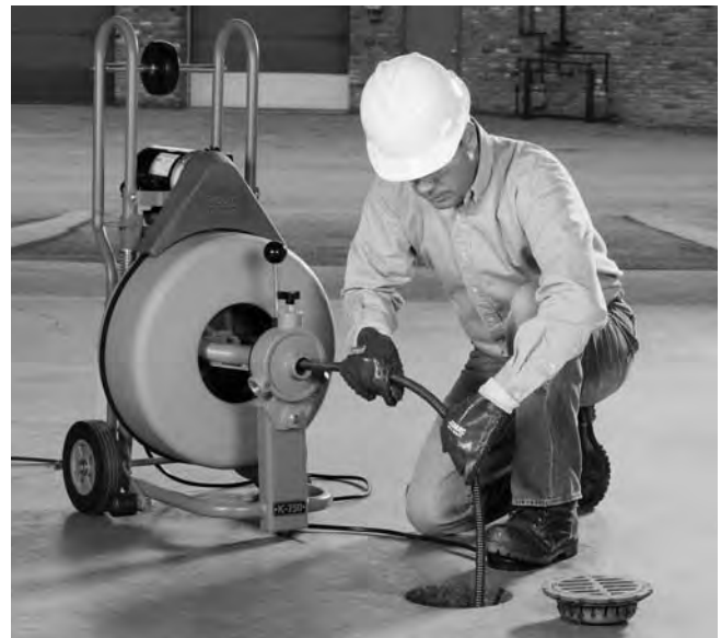
Figure 12 – In Operating Position, Manually Feeding Cable
