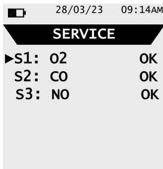
Messages on the state and calibration of the electrochemical sensors:
