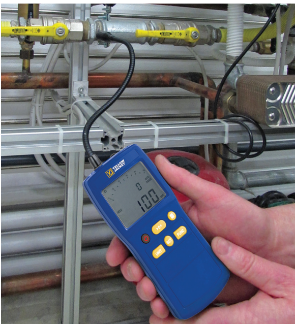
Displays Readings in PPM, % Vol. and % LEL
