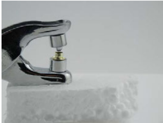
[Photo 3: Eyelet placed tube side up]
