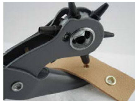
[Photo 2: Punch or cut a hole]
