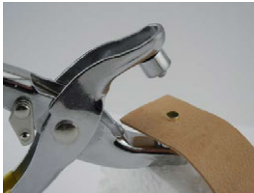
[Photo 4: Push eyelet through hole]
