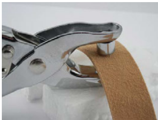
[Photo 5: Squeeze pliers firmly]
