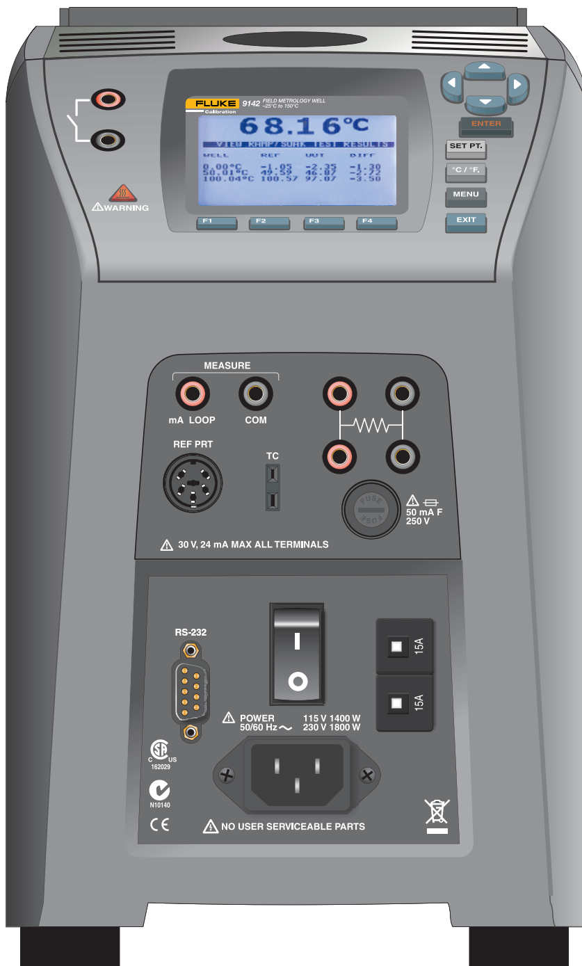
Figure 2 914X Field Metrology Well
