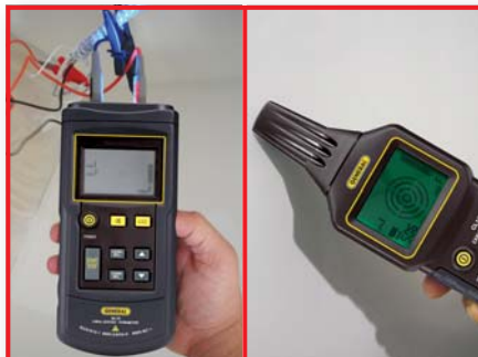
Tracing a cable behind a wall
