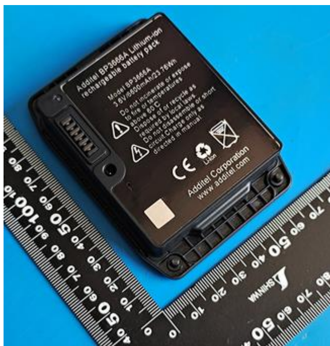
Additel BP3666A Lithium-ion rechargeable battery pack
