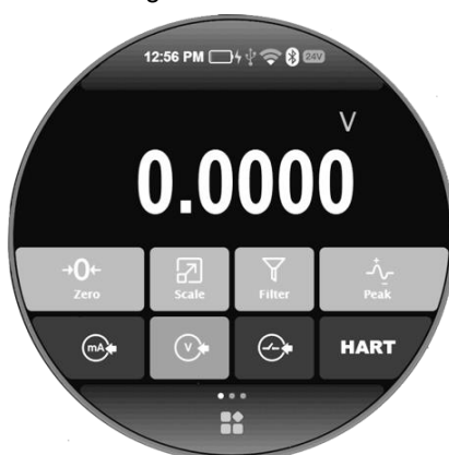
Figure 6 Electrical signal measurement function
