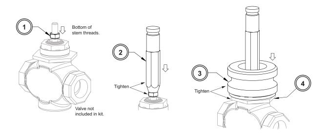
After the AV-821 adapter is installed, install the selected actuator and linkage (if required) according to the actuator installation instructions.
