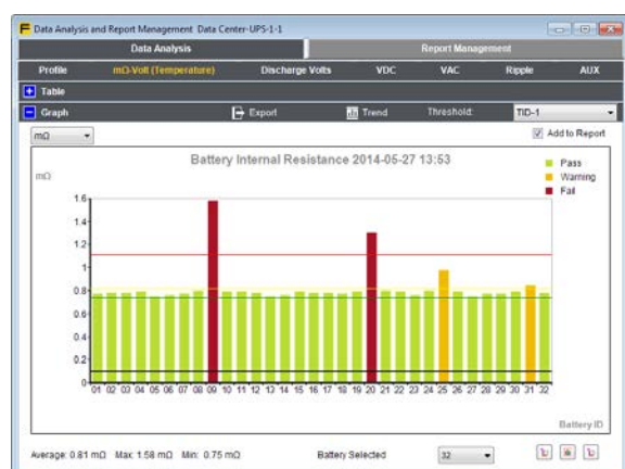
Histogram of a battery string with user defined threshold.
