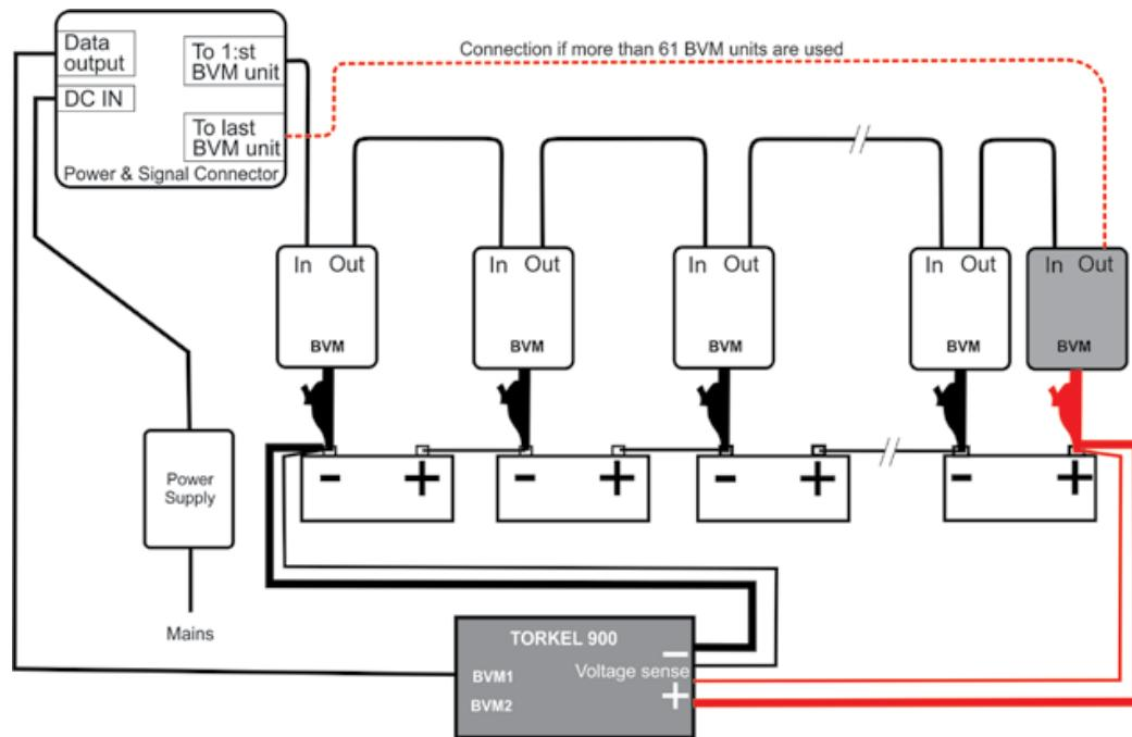
The BVM units must be connected following the battery cell sequence order. The red dolphin clip shall be connected to the most positive battery pole of the battery. The voltage over each BVM unit will be logged throughout the complete discharge test.
