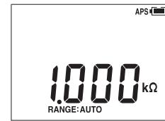
If resistance values of coils, including motors and transformers, measured with the auto-ranging fluctuate, select the range manually.
