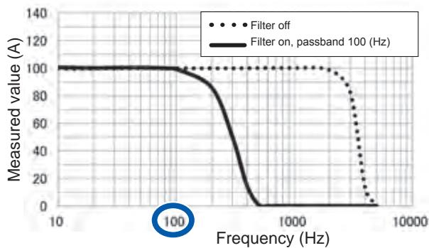
Disable the filter function when performing measurement of power supply frequencies in excess of 100 Hz, for example, on an aircraft or ship.
