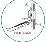
3 Connect the P200 oltage Probe to the measurement terminals of the instrument.
