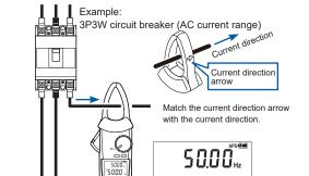
3 Clamp the instrument around the wire.
