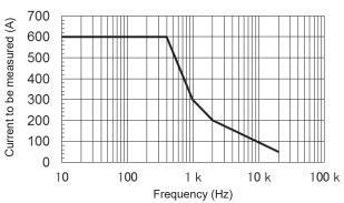
Inputting up to 1061 A of current is allowable for 1 minute or less. (66 Hz or less)
