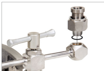
Remove the union nipple, nut, and o-ring...
