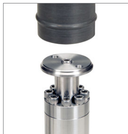
Remove the weight carrier tube...
