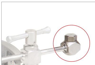
then replace with the plug and o-ring.
