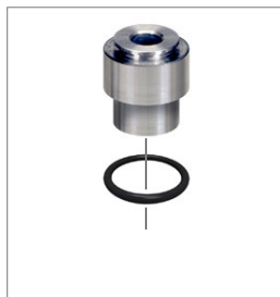
Remove the cylinder o-ring...
