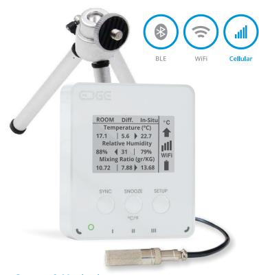
EDGE In-Situ is a high-precision data logger built for applications where understanding moisture dynamics between ambient and enclosed environments is critical.
