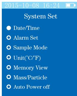
Press the **▲SET** button and the **ESC▼** button to select the menu option needed, then press button **START ENTER** to enter into the appropriate settings page.
