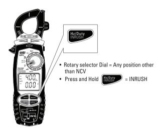
The UEi LRA Inrush is programmed to properly capture the starting current for compressor motors. Inrush current can be measured in any position of the rotary selector Dial.
