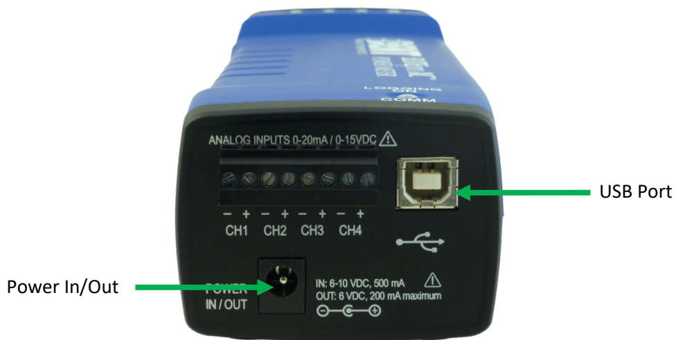
Power End Panel Connections
