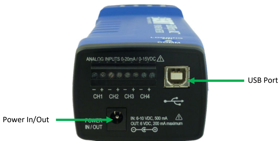
Power End Panel Connections
