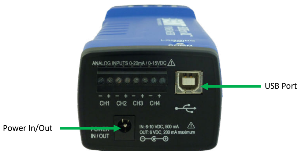
Power End Panel Connections
