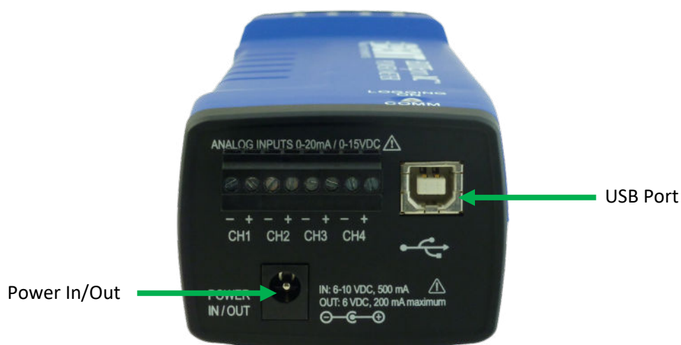
Power End Panel Connections
