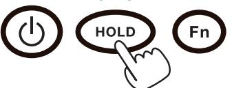
The HID function can be selected when the wireless communication function is enabled. Simultaneously pressing and holding the **HOLD** and **Fn** keys toggles the wireless communications function on and off. The display will show the
