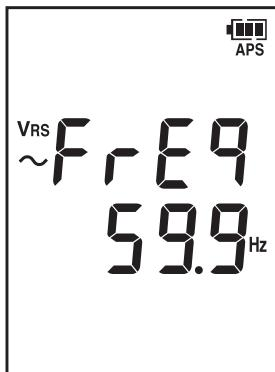
2 Check the measured value. (The frequency of the line-to-line voltage  $V_{RS}$  will be displayed.)
