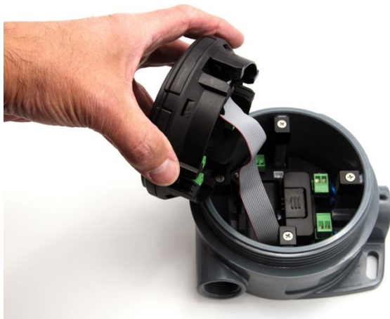
Options Board Mounted on the Bottom of Enclosure
