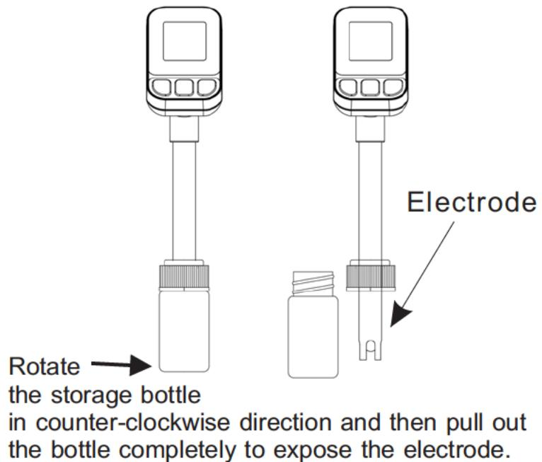
2. Dip the electrode into the test solution. Press "  $\textcircled{1}$  " to power on the meter and stir it to get a stable reading.
