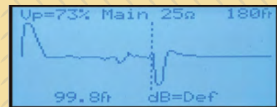
Graphical display of cable faults with digital indication of distance
