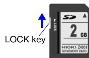
**4** Positioning the SD memory card with the top surface facing up, insert it into the slot in the direction shown by the arrow and push it all the way in.
