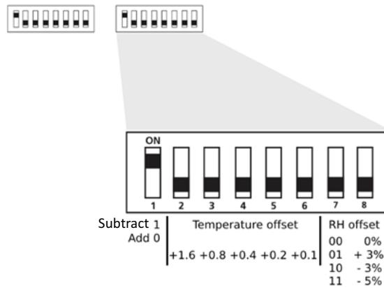
The first switch position is used to confirm if it is a positive (OFF) or negative (ON) temperature offset. Switches 2-6 are used to set a temperature offset value (see mapping above). Switches 7-8 are used to select a humidity offset to apply among the available values.
